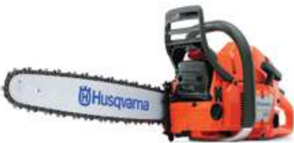
365 65.1cc - 3.4kW - 20" Bar - 6.0kg Magnesium crankcase | Three-piece crankshaft Quick-release air filter | LowVib® | Air Injection™ Smart Start®
