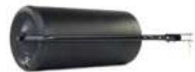
ROLLER - High density polyethene push or tow roller - 18" diameter - 36" working width (41.5" total width) - Weighs up to 164kg when filled with water - Can also be filled with sand
